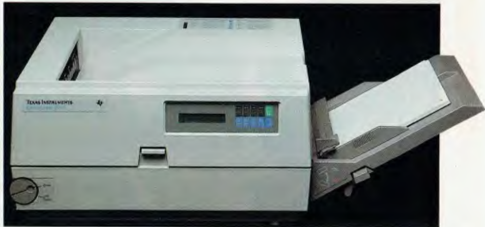
The Omnilaser 2106 from Texas Instruments has a small footprint, weighs only 17 kg, and has enough RAM to print out a full page of graphics – and includes PostScript.
